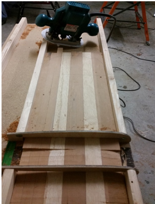
Shaping a flat board for a rudder section to a NACA shape using a router.
