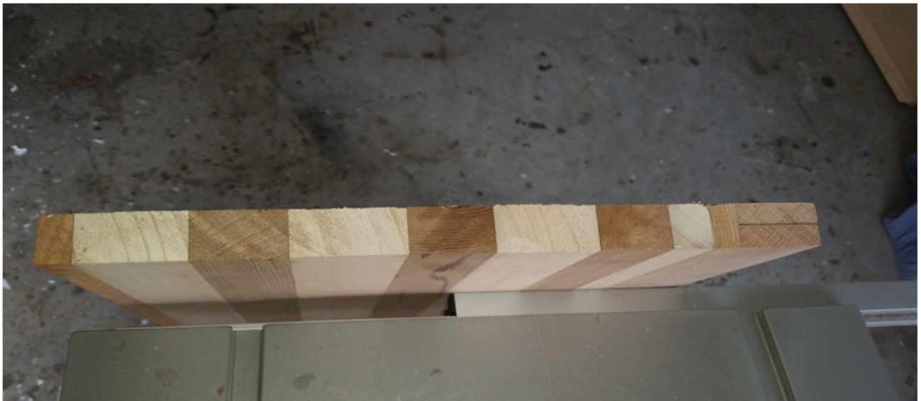
Flat centreboard section prior to shaping – note opposing end grain to prevent warping
