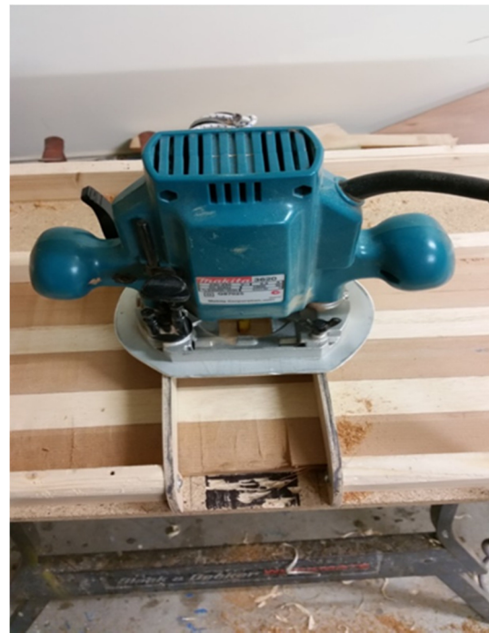
Shaping a flat board for a rudder section to a NACA shape using a router.
