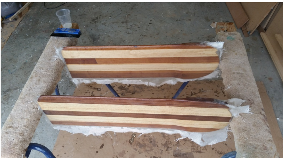
Sheathing Rudders using the 'drape over front edge' method.
