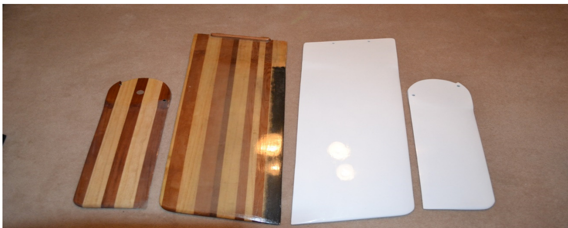
Finished products – Note external carbon fibre stiffening used on Centreboard trailing edge.
