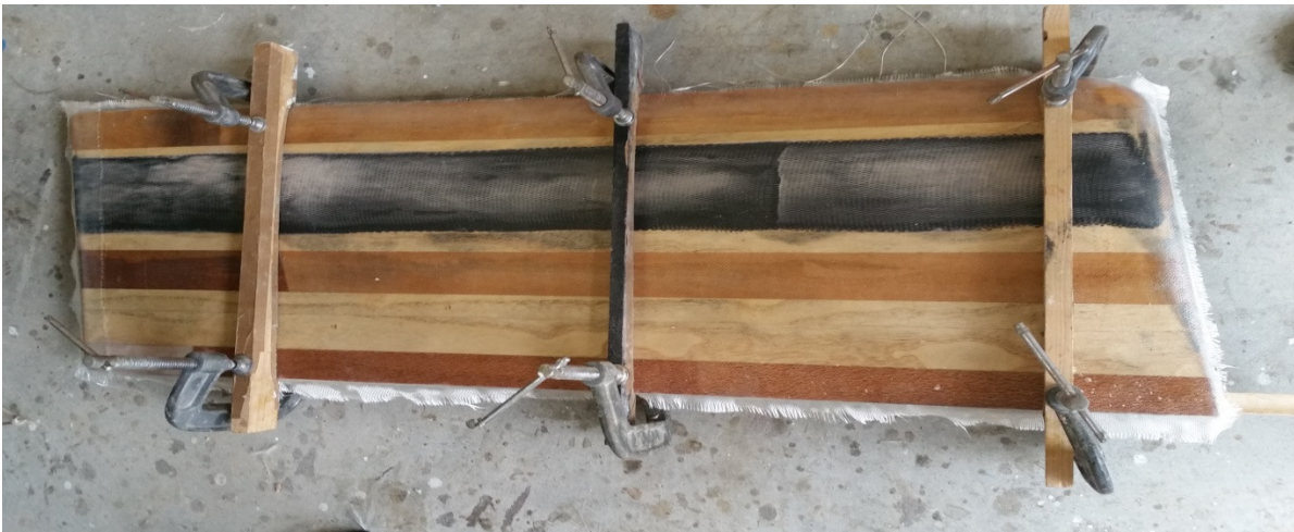
Centreboard sheathing process underway showing 100mm carbon fibre stiffening strip.
